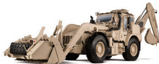
Built in Savannah, the fully armored JCB High Mobility Engineer Excavator (HMEE) is the world's toughest backhoe.
